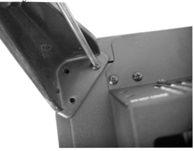
2. With use of a screwdriver, secure leg with the three screws provided (The screw is with the manual). Repeat the above for the other three legs.
